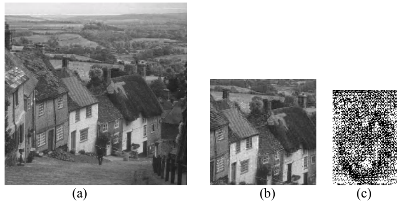
Fig. 8. Robustness provided by the proposed algorithm against cropping. (a) watermarked image (b) watermarked and cropping image, (c) extracted watermark image. (IPN logo)
